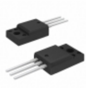
FQPF5N15 AMI Semiconductor / ON Semiconductor MOSFET N-CH 150V 4.2A TO-220F
