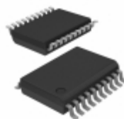
PIC16LF1826-E/SS Microchip Technology IC MCU 8BIT 3.5KB FLASH 20SSOP
