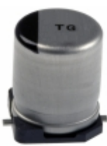
EEE-TG1A102Q Panasonic Electronic Components CAP ALUM 1000UF 20% 10V SMD
