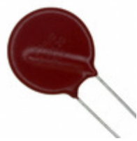
V575LU80B Littelfuse Inc. VARISTOR 889.5V 6.5KA DISC 20MM
