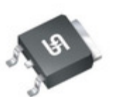
TSM6N50CP ROG TSC (Taiwan Semiconductor) MOSFET N-CH 500V 5.6A TO252
