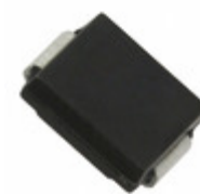
SMLJ45A Bourns Inc. TVS DIODE 45VWM 72.7VC DO214AB
