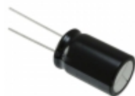
EEU-HD1H222 Panasonic Electronic Components CAP ALUM 2200UF 20% 50V RADIAL
