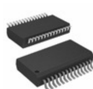
PIC24EP32MC202T-E/SS Microchip Technology IC MCU 16BIT 32KB FLASH 28SSOP
