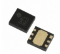
XC6121F629ER-G Torex Semiconductor Ltd IC WATCHDOG TIMER 6-USP
