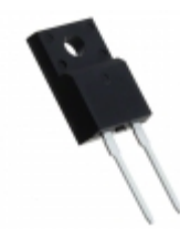
SCS206AMC Rohm Semiconductor DIODE SCHOTTKY 650V 6A TO220FM
