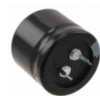
EET-ED2D821DA Panasonic Electronic Components CAP ALUM 820UF 20% 200V SNAP
