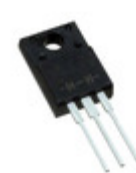
TSM10N80CI COG TSC (Taiwan Semiconductor) MOSFET N-CH 800V 9.5A ITO220
