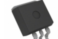
BD450M5FP2-CZE2 Rohm Semiconductor IC REG LDO 5V 0.5A TO-263-3F
