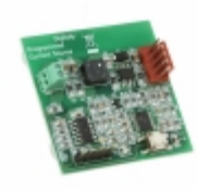
MCP1631RD-DCPC1 Micrel / Microchip Technology REF DES BATT CHARG OR LED DRIVER
