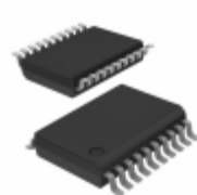
MCP1631HVT-500E/SS Microchip Technology IC REG CTRLR SEPIC 20SSOP
