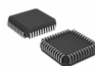
A3974SEDTR Allegro MicroSystems, LLC IC MOTOR DRIVER SER 44PLCC
