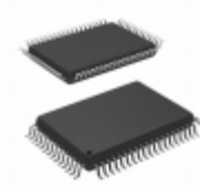
MB89P637PF-GT-5095 Cypress Semiconductor Corp IC MCU 8BIT 32KB OTP 64QFP
