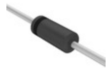
1N759A BK Central Semiconductor Corp DIODE ZENER 12V 500MW DO35
