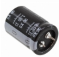
LGX2E561MELA35 Nichicon CAP ALUM 560UF 20% 250V SNAP
