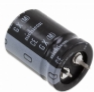
LGX2H680MELZ30 Nichicon CAP ALUM 68UF 20% 500V SNAP
