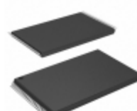
AT29LV1024-15TI Microchip Technology IC FLASH 1MBIT 150NS 48TSOP
