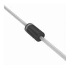
1N4735A-TAP Vishay Semiconductor Diodes Division DIODE ZENER 6.2V 1.3W DO41
