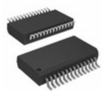
PIC16F18854-E/SS Microchip Technology IC MCU 8BIT 7KB FLASH 28SSOP
