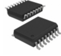
IS25WP128-RMLE-TR ISSI (Integrated Silicon Solution, Inc.) IC FLASH 128M SPI 133MHZ 16SOIC
