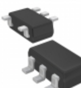
XC6123E426MR-G Torex Semiconductor Ltd IC WATCHDOG TIMER SOT-25
