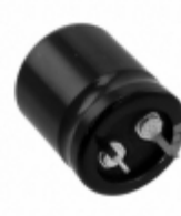
ECO-S1VP332BA Panasonic Electronic Components CAP ALUM 3300UF 20% 35V SNAP
