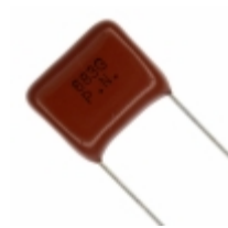
ECQ-P1H683GZ Panasonic Electronic Components CAP FILM 0.068UF 2% 50VDC RADIAL
