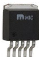
LM2575-3.3WU Microchip Technology IC REG BUCK 3.3V 1A TO263-5
