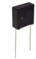
ECQ-E2W224KC Panasonic Electronic Components CAP FILM 0.22UF 10% 450VDC RAD
