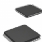
NUC230VE3AE Nuvoton Technology Corporation of America IC MCU 32BIT 128KB FLASH 100LQFP
