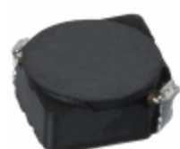
CDRH6D38NP-470NC Sumida America Components Inc. FIXED IND 47UH 950MA 155 MOHM
