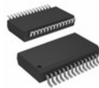
PIC16LF1788-E/SS Microchip Technology IC MCU 8BIT 28KB FLASH 28SSOP
