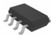
LTC2633HTS8-HZ8#TRMPBF ADI (Analog Devices, Inc.) IC DAC 8BIT DUL SPI I2C TSOT23-8
