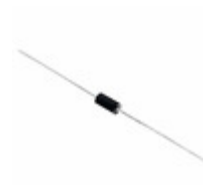
P6KE7.5CA Littelfuse Inc. TVS DIODE 6.4VWM 11.3VC DO204AC
