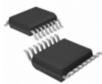
SQS16A1001JSLF TT Electronics/BI RES ARRAY 8 RES 1K OHM 16SSOP
