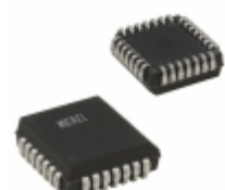
SY10H603JC Microchip Technology IC TRANSLATOR 9-BIT LATCH 28PLCC
