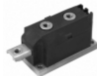
VSKHF180-12HK Electro-Films (EFI) / Vishay SCR MOD PWR 1200V 180A MAGNAPAK
