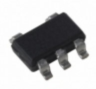
MIC5206-3.8YM5-TR Microchip Technology IC REG LDO 3.8V 0.15A SOT23-5
