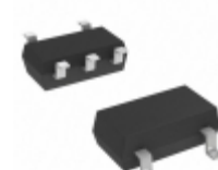
AN80L36RMSTX Panasonic Electronic Components IC REG LDO 3.6V 0.15A MINI5D
