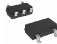
AN80L49RMSTX Panasonic Electronic Components IC REG LDO 4.9V 0.15A MINI5D
