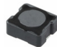
CDRH104NP-150MC Sumida America Components Inc. FIXED IND 15UH 2A 61 MOHM SMD
