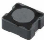
CDRH104NP-100MC Sumida America Components Inc. FIXED IND 10UH 2.4A 50 MOHM SMD
