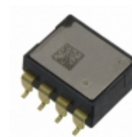
SCA620-EF1V1B-6 Murata Electronics ACCELEROMETER 2G ANALOG 8SMD
