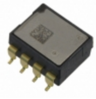
SCA620-EF1V1B-1 Murata Electronics ACCELEROMETER 2G ANALOG 8SMD
