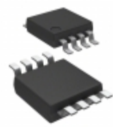
TC1173-5.0VUA Microchip Technology IC REG LDO 5V 0.3A 8MSOP
