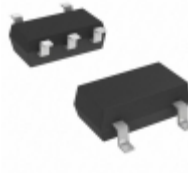
S-80953CNMC-G9PT2G SII Semiconductor Corporation IC VOLT DETECTOR 5.3V SOT23-5
