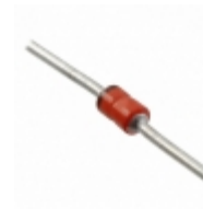
JANTX1N3016D-1 Microsemi Corporation DIODE ZENER 6.8V 1W DO41
