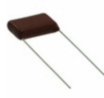
ECQ-E6124KFB Panasonic Electronic Components CAP FILM 0.12UF 10% 630VDC RAD
