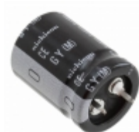
LGY2Z391MELZ Nichicon CAP ALUM 390UF 20% 180V SNAP
