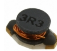
SDE6603-680M Bourns Inc. FIXED IND 68UH 400MA 860 MOHM
