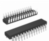
PIC16C57-RCI/P Microchip Technology IC MCU 8BIT 3KB OTP 28DIP
