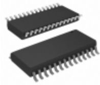
PIC16C57-LPE/SO Microchip Technology IC MCU 8BIT 3KB OTP 28SOIC
