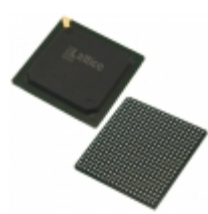
LFE3-35EA-6LFN484C Lattice Semiconductor Corporation IC FPGA 295 I/O 484FBGA
