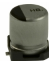
EEE-HP0J100R Panasonic Electronic Components CAP ALUM 100UF 20% 6.3V SMD
